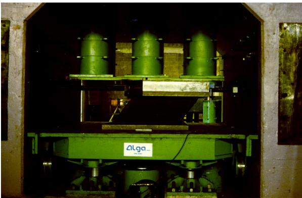
Fig. 10: Combined vertical and horizontal load test on a HDRB for Corinth Canal Bridge
