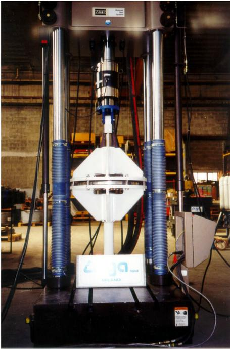
Fig. 32: Dynamic test of an electro-inductive damper of 250 kN capacity
