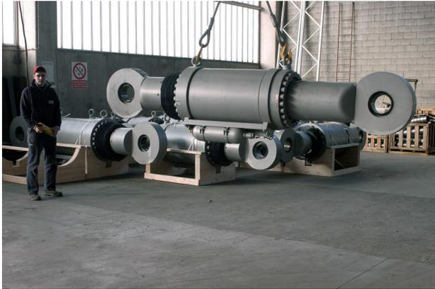
Fig. 30: STD of 12000 kN capacity and 800 mm stroke for the Paksey Bridge in Bangladesh
