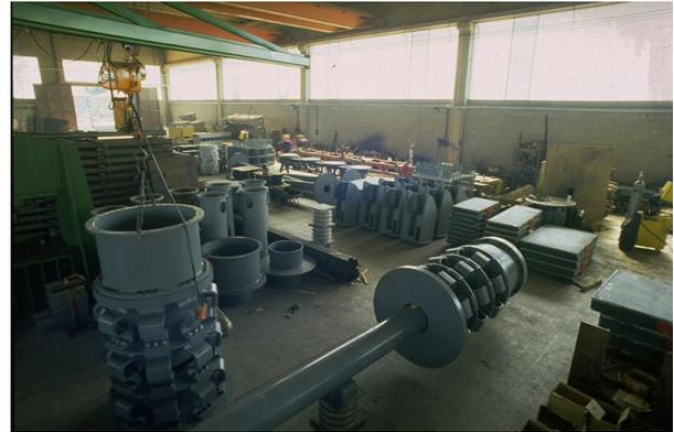
Fig. 16: The first hysteretic dampers utilised in Italy in 1980
